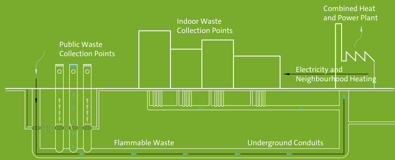
Waste collection with underground vacuum system (fig. 7)
