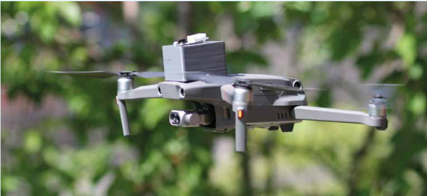
Use of an UAV for Remote Sensing Application: DJI Mavic 2 Enterprise with Thermal Camera (Fig. 17)
